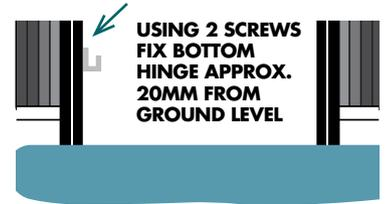
**3** From the bottom hinge measure up the post the height of the gate plus 25mm. Loosely install the top hinge so that it can slide up and down.
