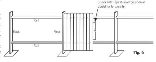
One easy way to achieve this, is to fix spaced palings on both sides of the rails. The high privacy gained by a normal close-butted paling fence would be reduced, but the spacing between palings on both sides can be adjusted to give adequate privacy with an advantage that cooling breezes can still penetrate.
